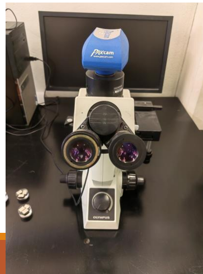
Microscopio óptico OLYMPUS GX-41. 50X, 100X. 500X
